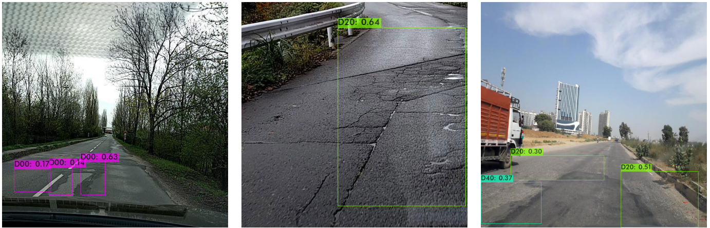
Fig. 1: Detection Results from a single YOLO-v4 model for different areas under varying lighting conditions and viewpoints in Czech, Japan, and India respectively.
