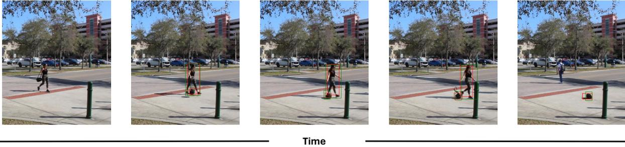
Figure 4. A person who drops a bag on the street is detected as an anomaly with our method. The detection starts with the action of "drop". After the object interaction ends, the dropped object continues to be detected as an anomaly. Ground truth labels and detection boxes are represented with green and red colors, respectively.
